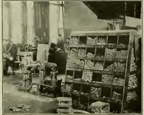
Fig. 12—Shears and Cabinet for Studs and Bolts.
